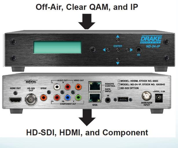
The *ND-24-IP* is ideal for broadcast and professional video applications where the demand is to decode a high quality live video signal from a wide variety of input sources. The *ND-24-IP* is a low cost professional video decoder that can decode an IP transport stream, off-air digital 8VSB channel or a program from a clear QAM source.
